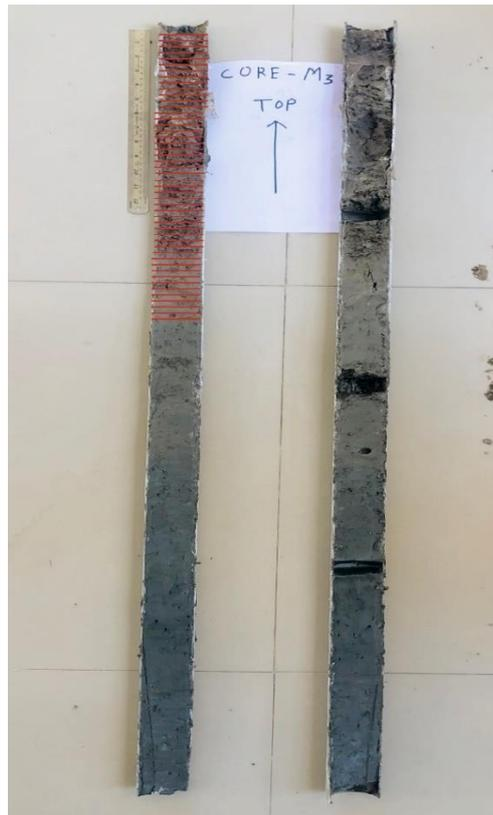
**Fig. 5.7:** Sediment characteristics and sampling at every 1 cm.
